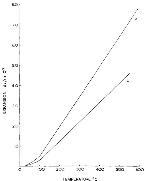
Figure 1 Expansion characteristics of the *a*- and *c*-axes of a  $\text{LiY}_{0.5}\text{Er}_{0.5}\text{F}_4$  single crystal. The data for the two measured *a*-axes were coincident and for the sake of clarity only one has been shown.
